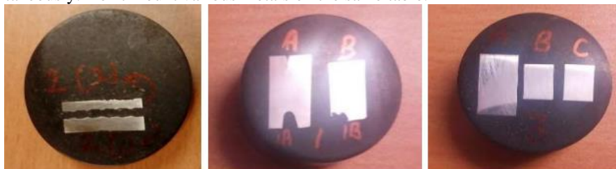
Figure: 4.37 Turbine blade specimens mounted in Bakelite
