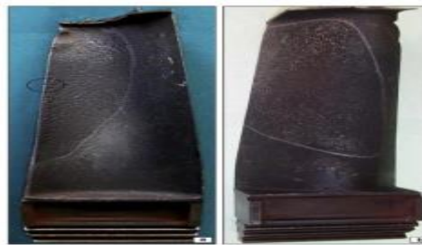
Figure: 4.17 General view of the blade number 3 showing corroded regions. (a) Concave surface. (b) Convex surface.
